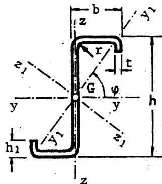
Luz ——  $l = 2,10 \text{ m}$ Acero —— F-24 ( $\sigma_F = 240 \text{ N/mm}^2$ )
