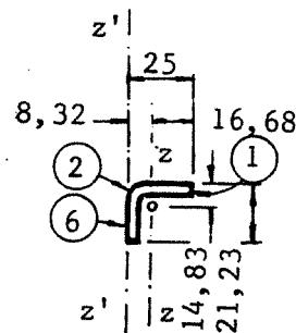
$$y_{Gs} = \frac{340,93 \text{ mm}^2}{40,97 \text{ mm}} = 8,32 \text{ mm}$$
