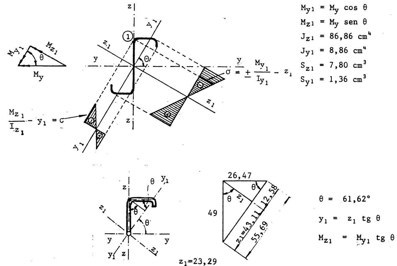
$$\sigma'_{cad} \geq \left| -\frac{M_{z1}}{J_{z1}} y_1 \right| + \left| -\frac{M_{y1}}{J_{y1}} \cdot z_1 \right|$$
